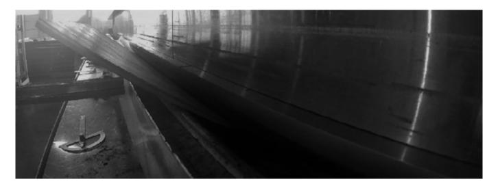
Swebor Armor™ 600 is an UHH protection steel which poses ability for cold forming. When cold forming Swebor Armor™ 600 personal safety precautions must be taken. We recommend bending of Swebor Armor™ 600 for the thickness.
